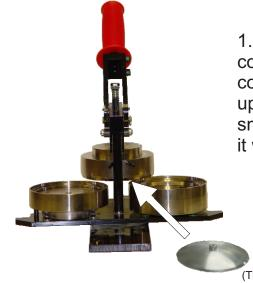
1. Before you begin assembly of your coaster button you must first place the coaster insert into the bottom side of upper die (flat side down). The insert will snap into place and it is magnetic so it will stay on its own.
