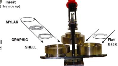
To remove the coaster insert, place the rod that came with the insert into the hole on top of the upper die.
