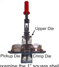
2. Prior to beginning you will need to examine the 1" square shells and determine which side of the shell has a burr, or a rough edge. You will only need to examine one shell in each box - the rest will be oriented the same way. Place the shell in the pickup die with the burr side facing down. Notice how the shell sits squarely in the die.
