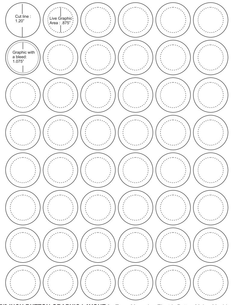
**7/8 INCH BUTTON GRAPHIC LAYOUT** for Tecre Manual or Electric Button Maker Machine LARGE CIRCLE IS CUT LINE. SMALL DASHED LINE IS RECOMMENDED MAXIMUM PICTURE SIZE.
